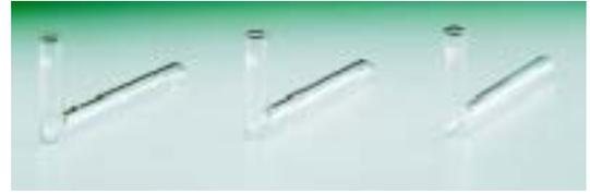
By inserting L-shaped culture tubes into the gradient block, an intermittent temperature-gradient incubation using a liquid medium can be performed. Up to 12 L-shaped culture tubes can be set at the same time.
