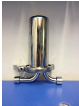
Photo of Steam Filter Housing with 1/2 NPT Connections. Flow through housing is bidirectional, so you can install the filter in any orientation.
