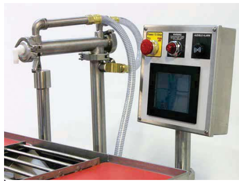
Water-jacketed depositing nozzle & pipe
