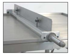
Adjustable Product Leveler: Set the desired depth and roll along side slab bars. It skims the top to a create an even batch
