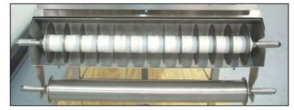
**<u>Rolling Drum Sizer</u>** Weighted drum to roll batch flat. Available in sizes to span width of table, or shorter lengths for smaller areas **<u>Table Cutter</u>** rolls along side slab bars and cuts entire length of batch. Side Saddles with Protective Cover for Table Cutter available **<u>Slab Bars</u>** Extra High or special sizes available as special order
