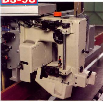
A large powerful air cylinder of dia. 25mm actuates a guillotine type cutter knife. Double springs, enable smooth and speedy cutter movement without noise.
