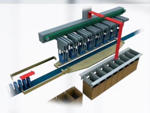
A solution for the continuous collating and positioning of plastic bottles to meet your specific requirements:
