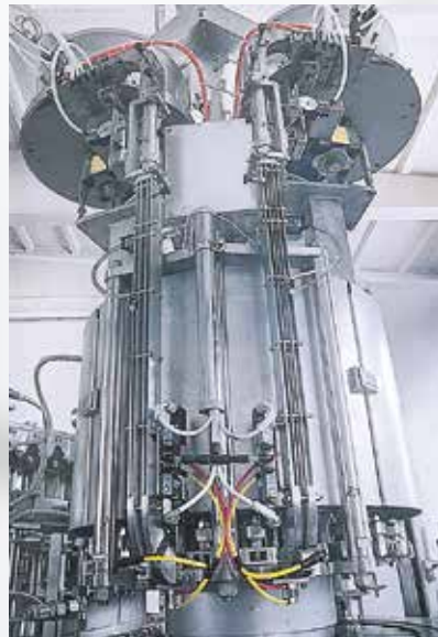
Crowner with double cap infeed chute
