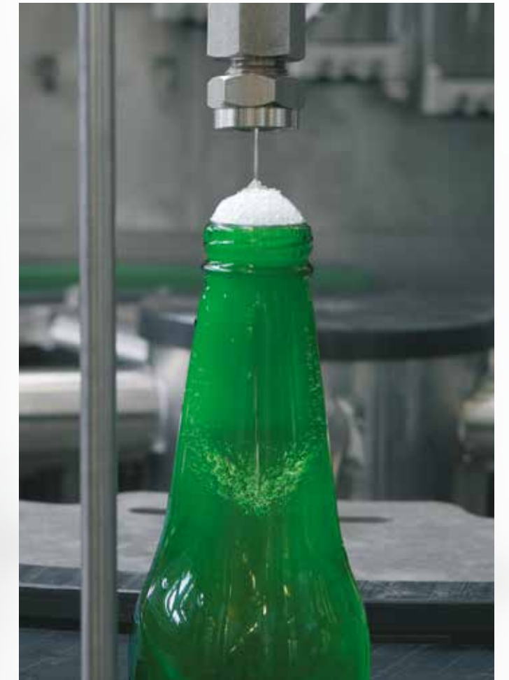
Detail of foaming system
