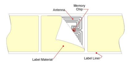
RFID tags are available in active, passive and semi-passive forms. Each type of tag transmits RF signals to be received and decoded by an RFID reader. Every tag has a unique identifier, allowing its signal to be differentiated from other RF tags.
