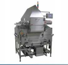
Wilevco's Rotary Atomization Spray Applicator utilizes patented "spinning disc" technology to maximize production yield.
