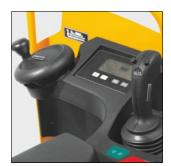
All drive and lift functions controlled by the multi-functional joystick on the ESE 220/320
