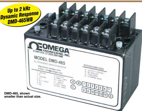
Dynamic Response: DMD-465: DC to -3 dB = 3 Hz DMD-465WB: DC to -3 dB = 2 kHz Max Output (2 kΩ Load): ±10 Vdc Output Impedance: 0.01 to 1  $\Omega$ Output Offset: -5 to 2V (DMD-465WB only) Gain Temp Coefficient: 200 ppm/°C Input Bias Current: 30 nA Input Impedance: 3000 M $\Omega$ Output Noise (RTO): @ gain = 100 DMD-465: 120 µVrms DMD-465WB: 1 Hz to 2 kHz = 2 mV Input Noise Line Frequency: 15 µV p-p Common-Mode Rejection: 90 dB @ gain 40, 100 dB @ gain 250
