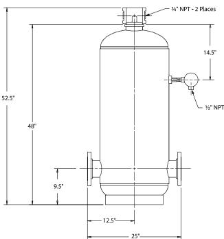
**Dimensions of 4" model shown** Consult the factory when certified engineering drawings are required. Dimensions shown are not suitable for construction or modifications.
