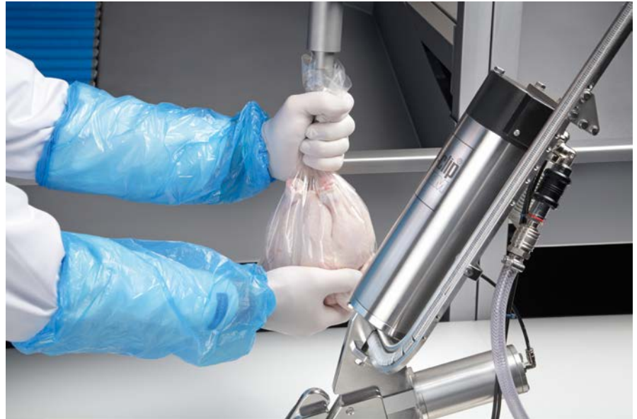
Vertical vacuum nozzle (pulling nozzle) in combination with the clipping machine EZ 600 of the Easy Clip Line®
