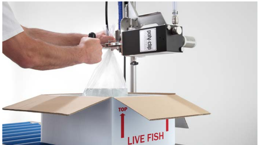
After filling with oxygen, the gate is closed and the clipping process is thus triggered.
