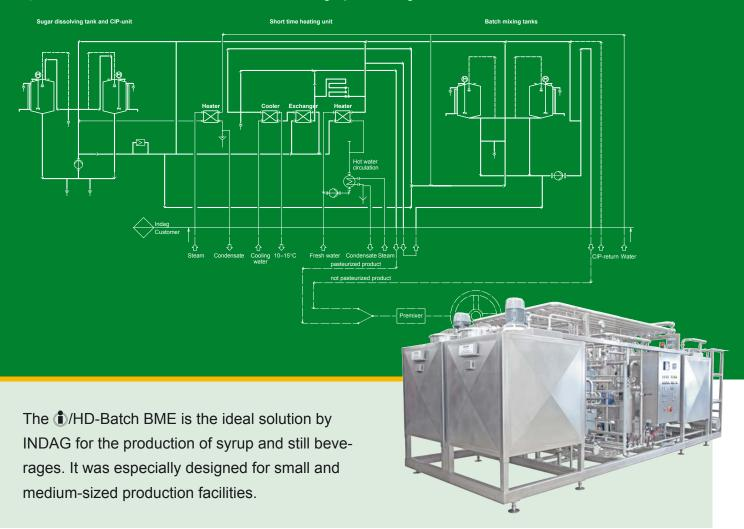
In the semi-automatic mode the Beverage Processing Module is able to produce about 1,500 to 2,000 liters syrup or beverages per hour. It is possible to combine the module with a premixer unit to manufacture final products out of syrup. Thus manufacturers can achieve an accordingly higher filling output. Especially for the small scale production the Beverage Processing Module offers a complete solution which covers all necessary features for the modern beverage production.
