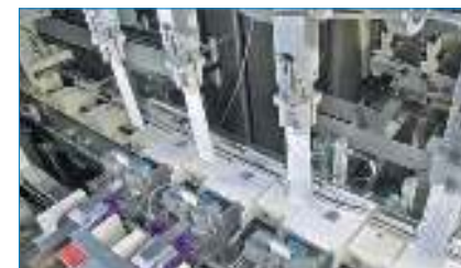
TLM system components (blank magazine, transfer unit and the TLM-F2 robot) remove four pre-glued blanks at a time and transfer them to the TLM conveying system.
