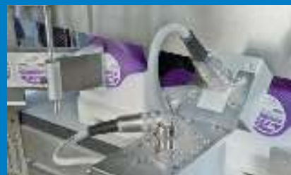
The round labels are positioned with millimetre accuracy. The labelling system from Weller prints the labels using the thermal transfer method and verifies them directly after the labelling process.
