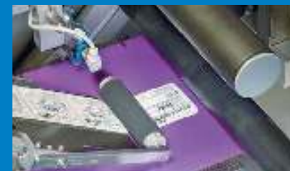
The primary packaging of the inhaler is labelled prior to the actual flow wrapping process in order to guarantee a crease-free label.
