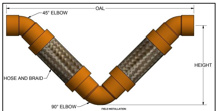
ASSEMBLY MATERIALS: HOSE/BRAID: BRONZE 90° ELBOWS: COPPER 45° ELBOWS: COPPER 1. FIELD CONNECTIONS USING BRAZING OR SOLDERING PROCESS SHOULD NOT USE A FLUX THAT IS CHLORINATED. FLUX THAT IS RESIDUAL ON THE INTERIOR AND EXTERIOR OF A HOSE THAT IS CHLORINATED WILL CORRODE AND CAUSE PREMATURE FAILURE OF THE STAINLESS STEEL AND VOID ANY WARRANTY.
