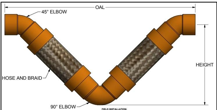
ASSEMBLY MATERIALS: HOSE/BRAID: BRONZE 90° ELBOWS: COPPER 45° ELBOWS: COPPER 1. FIELD CONNECTIONS USING BRAZING OR SOLDERING PROCESS SHOULD NOT USE A FLUX THAT IS CHI ORINATED. FILIX THAT IS RESIDIAL ON THE INTERIOR AND EXTERIOR OF A HOSE THAT IS
