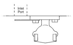
Baffle Arrangement used on 40 mm:-FT 10, FT 46 FT 43, FT 44 and FT 47 (horizontal only)
