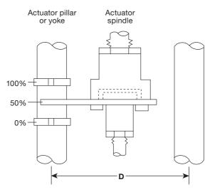
Fig. 4 Pillar/voke spacing, showing 50 % travel.
