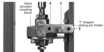
Fig. 2 Close-up of sliding pin holder fitted to valve coupling.
