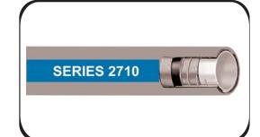
An exceptionally versatile sanitary hose designed to handle a wide variety of products and application requirements (Meets 3-A standards, USDA requirements and is FDA compliant). The specially compounded tube is engineered to handle high temperatures, will not impart taste or odor and is <u>highly resistant to common CIP solutions</u>. Manufactured on polished chrome mandrels, our mirror finish tube resists bacteria growth, while providing excellent flow rates.
