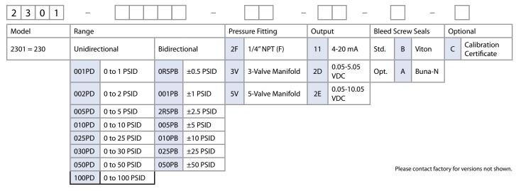
Ordering Example: 2301005PD2F11B = Model 230 0 to 5 PSID unidirectional, 1/4-18 NPT Male fitting, 4 to 20 mA Output, and Viton/Silicone Seals. 2301005PD3V11B = Model 230, 0 to 5 PSID unidirectional, 3-Valve Manifold, 4 to 20 mA, Output, and Viton/Silicone Seals (Assembled w/3- Valve Manifold).
