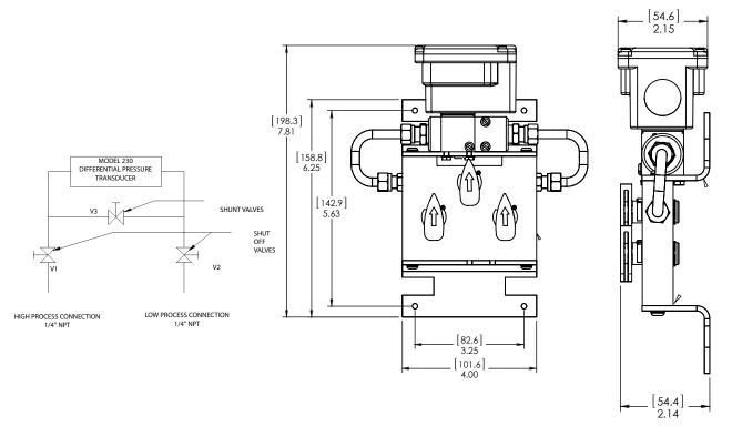
For differential pressure measurements at high line pressure (350 PSIG max), it is recommended that the pressure sensor be installed with a valve in each line, plus a shunt valve across the high and low (reference) pressure ports as shown.
