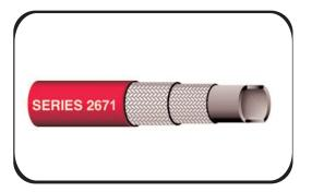
This is a heavy duty hose for high pressure water booster service on fire engines. Tube and cover compounds resist abrasion and weathering. Tough yet flexible, for resistance to flexing and surge loads. Meets NFPA 1961 requirements under current RMA specifications. Meets or exceeds UL92 requirements for 800 PSI Booster Hose. Hose is non-conductive.
