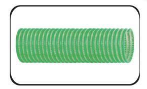
Designed to be Biofuel compatible, this specially formulated polyurethane drop hose handles gasoline, ethanol (up to E98), diesel and biodiesel (up to B100 meeting ASTM D6751 criteria). The polyurethane construction is non-permeable, lighter weight than conventional TPR/Rubber hose, and has superior sub-zero flexibility. The clear side wall of **Series 1985** allows for easy inspection of material flow and the external helix provides for easy drag.
