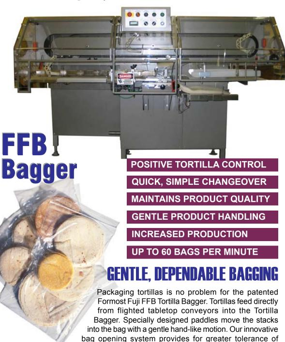
The FFB Bagger is compact, durable and carefully engineered for trouble-free operation. It will save maintenance costs, too. All parts are readily accessible
