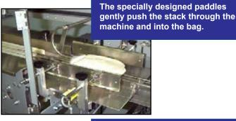
The innovative bag opening system prepares each bag for insertion of the tortilla stacks.
