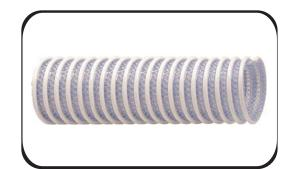
Reinforced, flexible heavy duty PVC food grade suction hose designed for handling various food products. Braided reinforcement will accommodate higher working pressures while maintaining excellent flexibility and light weight. Typical applications include processing wine, beer, paste food, dairy and liquid foods. In compliance with criteria of 3-A, FDA, USDA.
