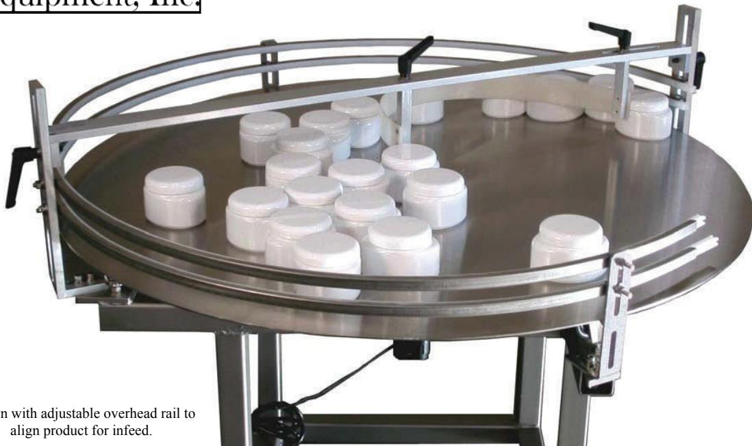
Shown with adjustable overhead rail to align product for infeed.
