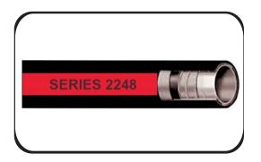
Series 2248 is designed for heavy-duty service in the transfer of petroleum products up to 50% aromatic, including leaded and unleaded gasoline, oil, and diesel fuels. Ideal for applications where an extremely lightweight, flexible hose with a high working pressure and small bend radius is required. The specially formulated **Carboxylated Nitrile** cover is designed for **superior abrasion resistant** applications.
