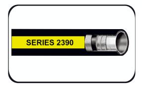
This hose is specifically designed to convey hot air at 350°F continuously in the process of loading/unloading dry materials in plants or transport vehicles. The hose transfers hot air from the compressor to the storage bin/cargo bay to propel bulk product. The specially formulated EPDM tube and cover offer excellent resistance to heat as well as to weather and ozone.
