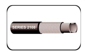
Designed to handle both water and oil based paints in medium pressure applications. The Nylon 11 tube will handle ketone solvents, lacquers, thinners and paints with high aromatics, as well as many chemicals. Very flexible for ease of handling.
