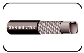
An economical and versatile general purpose hose. Excellent for air and water service, as well as many agricultural chemicals including Lasso® herbicide. EPDM tube and cover resists heat, sunlight, ozone and weathering. This hose exceeds ARPM Class C medium oil resistance requirements. Suitable for applications such as oil mist lubricating air lines, but **NOT** suitable for the transfer of petroleum products.
