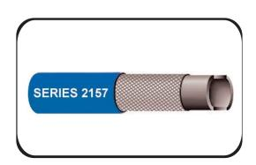
Economical and versatile general purpose hose. Excellent for air and water service as well as many agricultural chemicals including Lasso® herbicide. EPDM tube and cover resists heat, sunlight, ozone and weathering. Suitable for applications such as oil mist lubricating air lines, but **NOT** suitable for the transfer of petroleum products.
