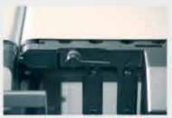
Simple, toolfree belt removal via cams for the simplest possible cleaning with the machine running (cleaning program).
