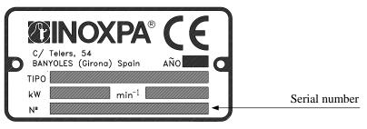
Figure 3.1: Characteristics plate.
