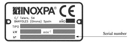
Figure 3.1: Characteristics plate.
