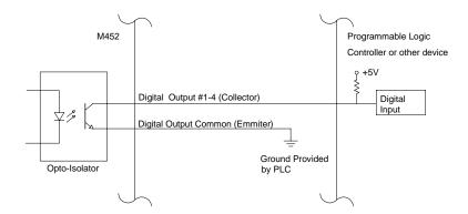
Figure 4-2: Digital Output Connections
