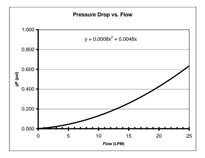
Figure 2-2: Pressure Drop vs. Flow (High Purity Version)
