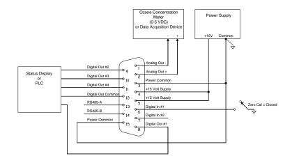
**Figure 4-1: Electrical Connections**
