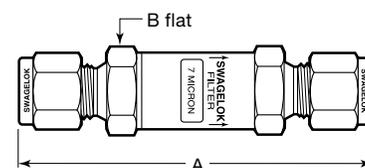
Dimensions shown with Swagelok tube fitting nuts finger-tight.
