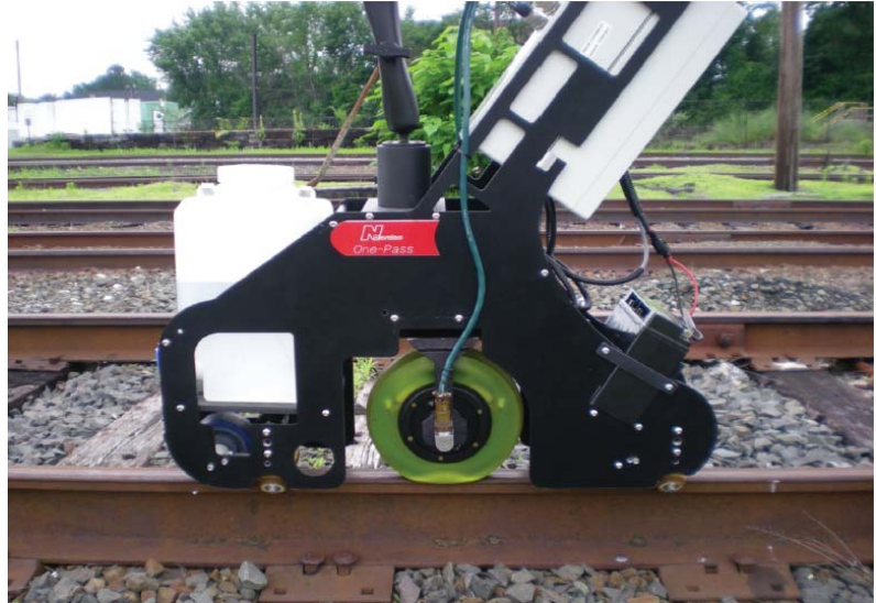
One Pass - Ultrasonic Rail Inspection System
